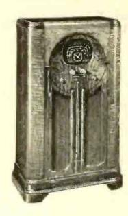
MODEL 670C - "Automatic Maes-MODEL 670C — "Automatic Maestro" model; 9 tube, 11 tube performance, All-Wave American, Police and Foreign, plus U. S. weather band, improved superherodyne Console. Range: standard hroadcast and police 525 to 1890 Kilocycles; police and short wave 1800 to 6000 Kilocycles; short wave 6000 to 18500 Kilocycles; and long wave U. S. weather band 150 to 375 Kilocycles.
