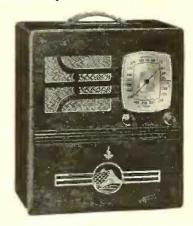
★ Six-tube battery portable superhet. Operates from self-contained dry batteries—weight 26 pounds. Battery conservatively estimated at 150 hours' service. Permo-magnetic speaker—3gang condenser. Sturdy walnut cabinet. Model H-137—list \$49.95 with batteries.
