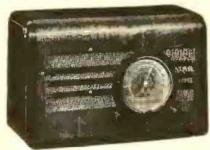
Model 87—dual band AC-DC superhet with 7 tubes including ballast. Range—550-1600, 5500-15,500 kc. 2-gang tuning condenser—4½-inch dial with planetary drive. Six-inch dynamic speaker. Size 10 x 16 x 6% inches walnut cabinet. List \$29.95.
