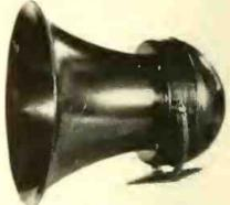
\* Speaker horn for use with ten-inch dynamic speakers—projects sound in desired direction thereby saving on amplifier power. Constructed of spun brass with black enamel finish. Mounted on searchlight type bracket. 18-inch bell and 17 inches long—weight 5 pounds. Model 42. Operadio Mfg. Co., St. Charles, Ill.—Radio Today
